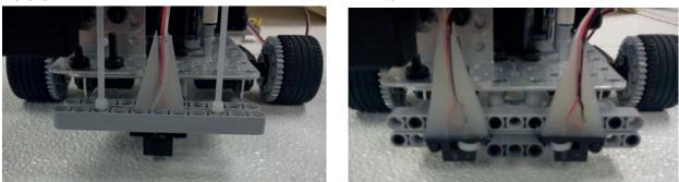
Our original sensor mount had only one tophat sensor, however it wasn't able to follow the line on the ramp. In order to fix this we altered the mount to have two tophat sensors. With the two tophat sensors it would be able to better correct itself on the ramp as well as determine when it reaches the top of the ramp. We will continue to test in a similar manner to how we did with the one tophat, just with the new code and hopefully better results.
