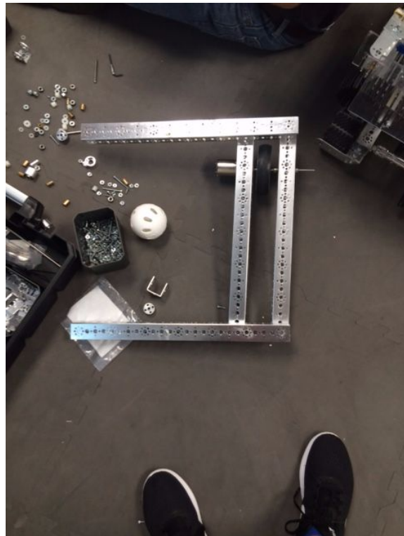
Above the chassis prototype started to help us test the wheel configuration. There will be discussion regarding the final motor and wheel placement in the design.
