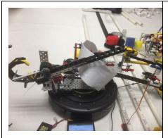
On our create we have a claw attached to an igus chain, allowing it to change elevation and reach the poms on the terrace. Initially, we considered using a standard claw on a rod attached to a fulcrum. We ended up not going with this design as when the claw was raised it stopped being parallel to the ground unlike with the igus chain.
