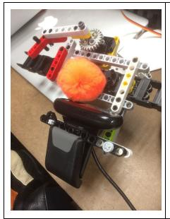
We sandwiched the base flap of the camera between two lego beams which were connected by axles to secure it. We alternatively considered putting lego beams around the head of the camera itself. We ended up not going with this strategy as it was looser than the alternative, meaning that the poms would have always been in different locations in the camera's view.
