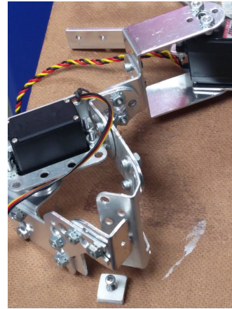
Figure 22.1 and 22.2 : Relic grabber and its placement on the extrusions itself
