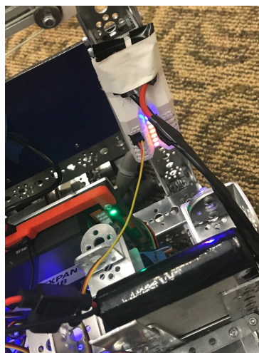
Figure 30.3 and 30.4 :Finished Glyph arm system and the servo power module
