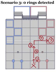
1. Move forward ~12 in.; rotate ~5 degrees to detect rings and rotate back
