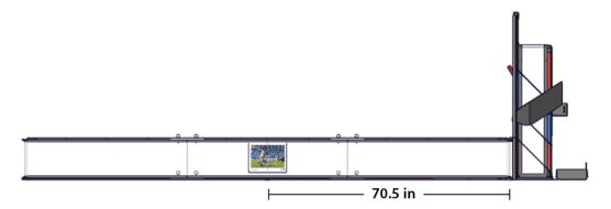
• The Navigation Image horizontal center line should measure 6.375 inches to the floor (5.75 inches from the top of the tile).
