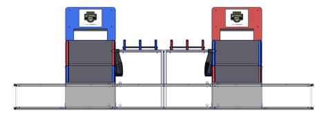
The Power Shot Assemblies should be placed as close together as possible and secured together with two cable ties. One at the top and one at the bottom of the assemblies.
