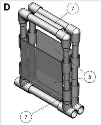
Note 1: Acrylic window (or substitute can be attached using duck tape, foam mounting strips (like commands strips), or other. We recommend white duck tape as that is what we will likely use for tournaments. The best method for attaching them is to lay one window down on top of PVC couplers and fasten with tape.
