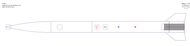
Apogee: 386 m Max. velocity: 109 m/s (Mach 0.32) Max. acceleration: 114 m/s<sup>2</sup>
